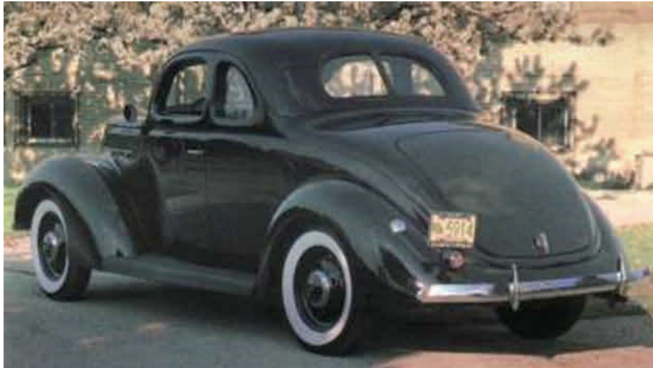
The rear view of the 1937 Ford Model 74 shows the sharply sloping trunk lid
