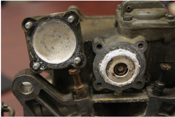
Ethanol damage to a carburetor. Photo by Tom Shaw, courtesy SEMA
