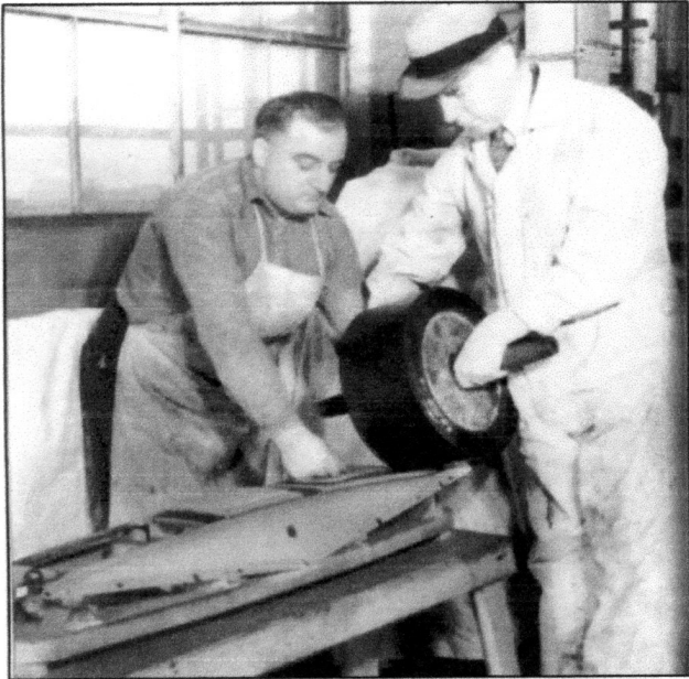
Skilled craftsmen apply the woodgrain to a 1939 dashboard. The fedora and tie are a nice touch!
