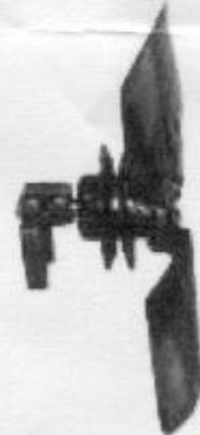
The completed fan-hub-shaft assembly with mounting bracket
