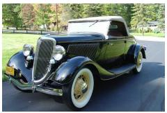
The '34 Roadster is a full restoration of a body with no rust-out. It came with NOS running boards (which had to be recovered), two NOS rear fenders and a good used grille. The body was done on a rotator, completely sand blasted and epoxy primered. The radiator is new using original frame and top and
