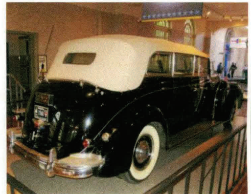
Rear view of 1939 Lincoln "Sunshine Special" on display at the Henry Ford Museum - note the platforms and hand grabs for Secret Service agents
