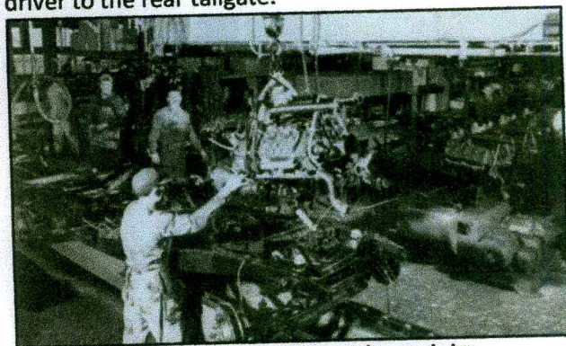
A 1940 chassis gets its engine and transmission.
