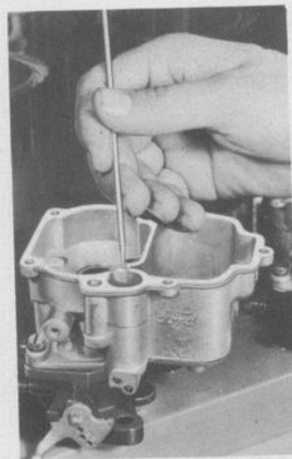
Figure 99—Removing Check Valve Retainer
