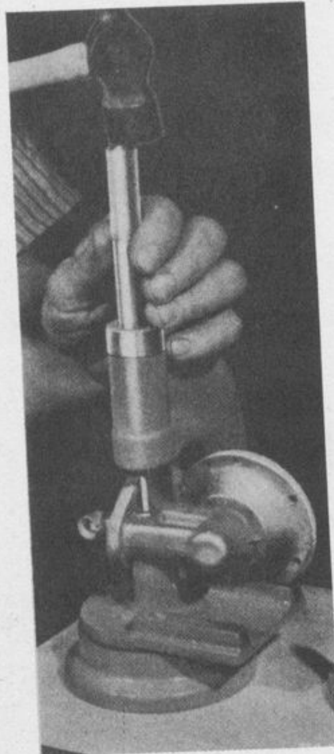
Figure 174—Fixture for Removing Rocker Arm Pin
