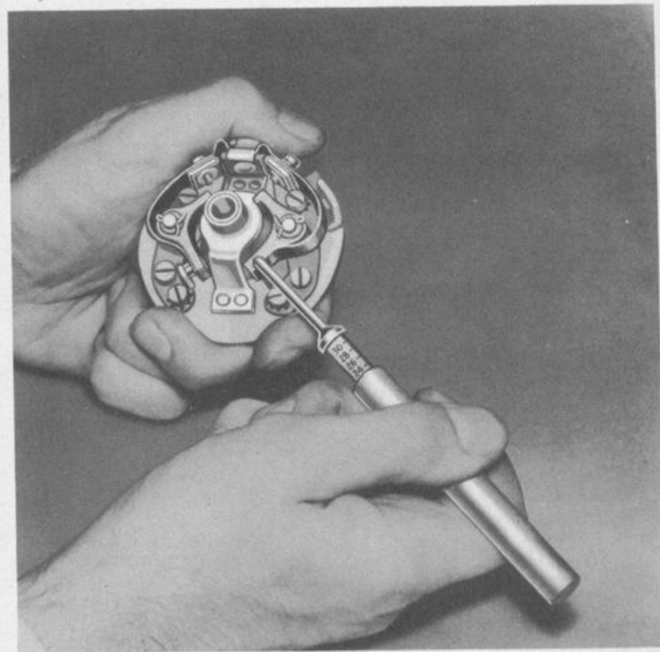
Figure 212—Checking Breaker Arm Spring Tension
