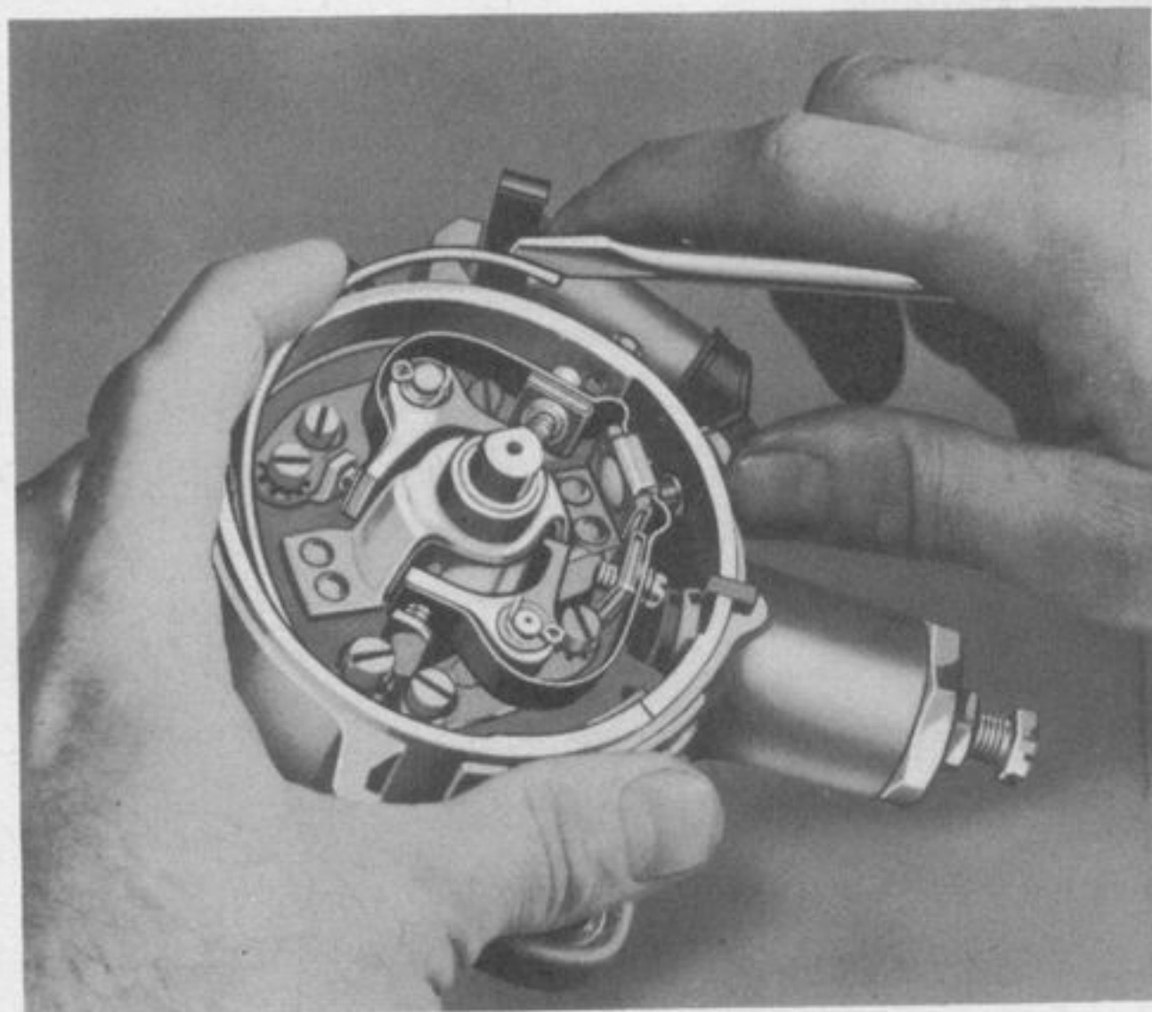
Figure 213—Installing Distributor Base Spring
