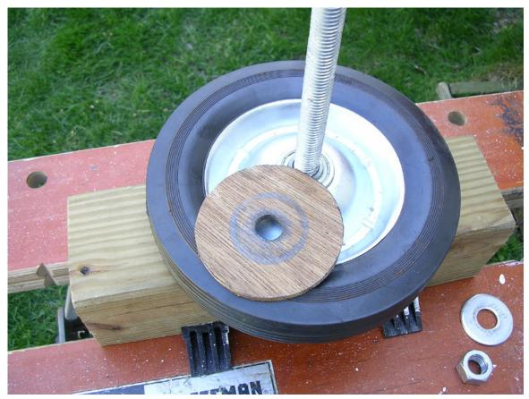
The centering piece for the rim is held in place with another 5/8" flat washer and two 5/8" hex nuts. The hex nuts are locked together, and then backed off so that the wheel spins freely and without any wobble. I sprayed a little WD40 at the base of the two locking nuts and the flat washer to help. I also sprayed white lithium grease into the wheel bearings of the 8" wheel.
