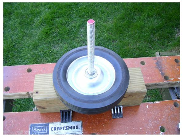
You can do a pretty good job of centering the wheel to be painted by just using the hub bolthole pattern as a guide, but I felt that a more secure centering mechanism was needed. I marked and cut a circle out of 1/4" plywood that just fit into the wheel hub hole, and drilled a 5/8" hole in the center.
