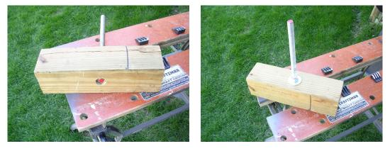
The base assembly would now clamp into the Workmate. The 8" wheel would rest on the hex nut, and the wheel rim and tire to would rest on top of that.
