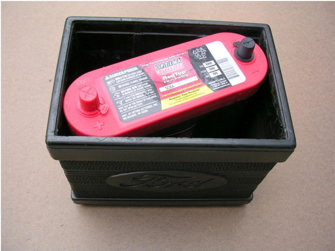
Figure 5 - Optima positioned in case. Positive terminal goes to the Ford script side.
