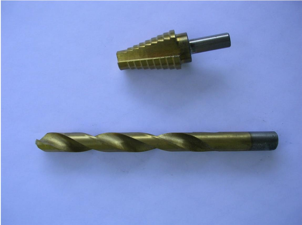
**Figure 13 - 1/2" drill for pilot hole, and 1" step drill used for holes for battery caps and terminal posts**
