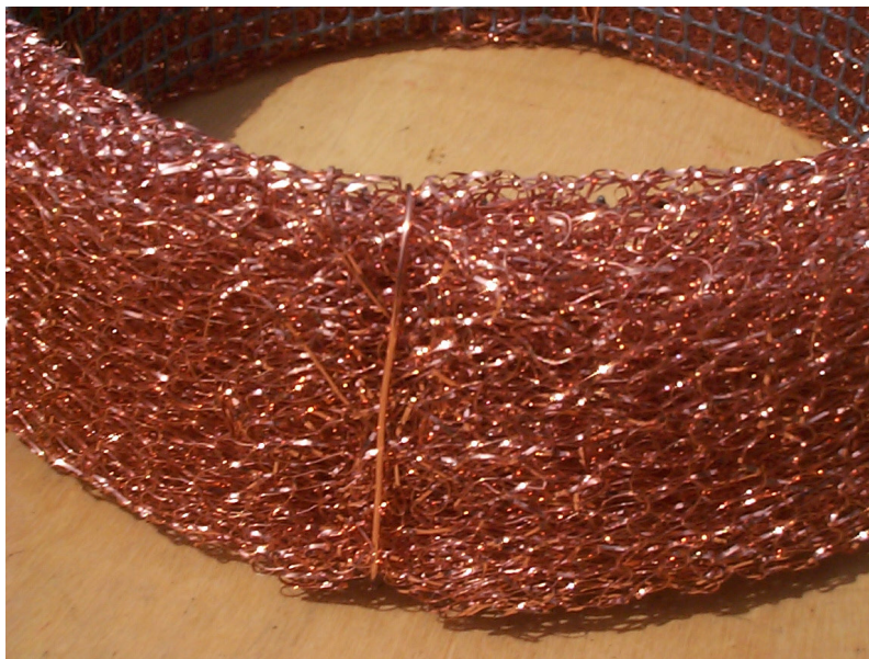
Figure 7 Top wire bent down & around to hold the wound mesh.
